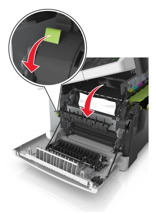
**4** Hold down the fuser cover, and then remove the jammed paper.
