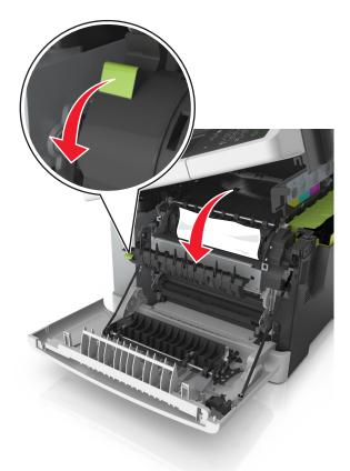
**c** If there is a jammed paper in the fuser, then hold down the fuser cover, and then remove the paper.
