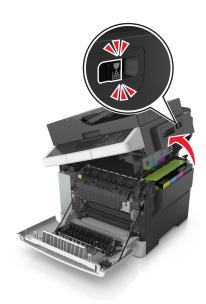
**3** Pull the green lever to open the fuser cover.
