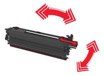
**11** Remove the red packing strip and the attached fabric from the developer units.
