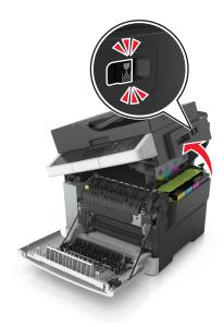
3 Remove the toner cartridges by lifting the handles, and then gently pulling them away from the imaging kit.
