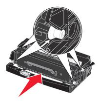
6 Install the print cartridge assembly into the printer by aligning the green arrows on the guides of the print cartridge assembly with the green arrows on the tracks in the printer and pushing the print cartridge assembly in as far as it will go.
