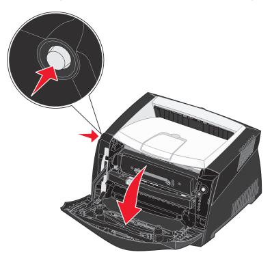
2 Pull the print cartridge assembly out of the printer by pulling on the toner cartridge handle.
