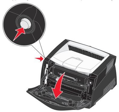
**3** Remove the print cartridge assembly out of the printer by pulling on the toner cartridge handle.
