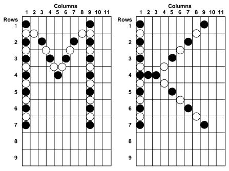
When a diagonal line intersects a vertical line at a point other than the end of the vertical line, you should specify a horizontal dot at the intersection to improve character appearance. This ensures that the character is acceptable in Draft.
