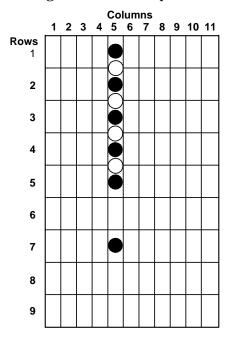
The solid dots must be specified in the font. Hollow dots are generated by the printer.
