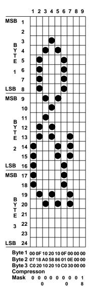
This example shows the design for the ampersand character (ASCII 38) from the All Characters chart. This character design does not have any occurrences where extra dots can be added, resulting in a column being identical to its predecessor. For instance, column 4, row 4, could be turned on because it would automatically be turned off during printing, but other bits in column 4 are different from column 3, which means no compression can occur. Column 9 is identical to column 8 (blank).
