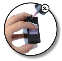
Now insert the syringe inclined into each opening. Slowly and carefully squeeze the ink into each ink chamber, until just under the openings. If some ink emerged from the nozzles, simply draw up a small quantity of ink from the chamber into the syringe. To make sure that you inject the right colour into the correspondent colour chamber while refilling, start to identify each colour chamber, inserting a toothpick through the openings. Replace the label afterwards.
