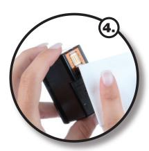
Finally clean the area around the nozzles with a tissue, until these are clearly visible. You may now insert the refilled cartridge into the printer.
