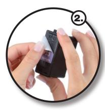
First remove the label from the upper side of the cartridge und bore refilling holes. To do so, use the supplied tool to enlarge the 3 existing openings.
