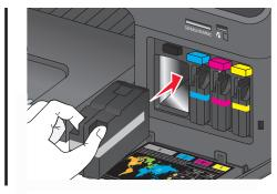
**Note:** Install the new ink cartridges immediately after removing them from the packaging to avoid exposing the ink to air.
