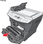
Warning: Do not leave the print cartridge assembly exposed to direct light for an extended period of time.
