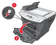
**2** Pull on the handle to remove the print cartridge assembly.
