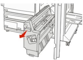
**7** Lift the inside cover. If the paper is jammed in the rollers, rotate Knob G8 clockwise, and then remove the jammed paper.
