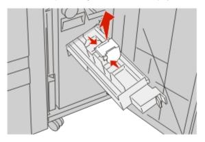
Remove the jammed staples, and then place the staple cartridge into the stapler.
