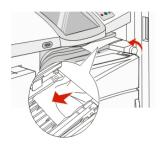
**Note:** If the paper jam on the right is difficult to remove, rotate the knob clockwise.
