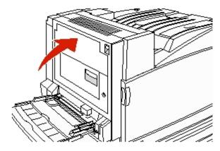
**5** Pull the multipurpose feeder down, and then open Door B.
