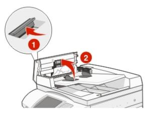
**3** Raise the sheet guard, and then remove any jammed paper.
