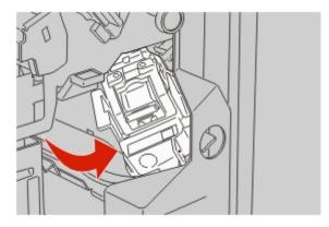
**3** Lift the lever, and then remove the staple cartridge.
