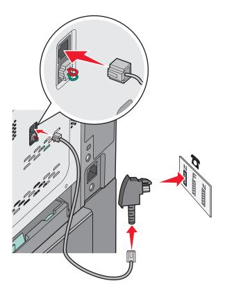
**3** Connect the adapter into the N slot of an active analog telephone wall jack.
