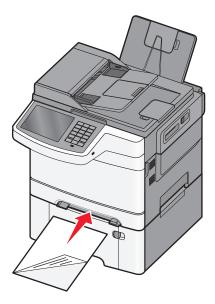
**Note:** Align the long edge of the sheet so that it is flush with the right side of the manual feeder.
