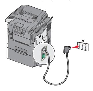
4 If you would like to use the same line for both fax and telephone communication, then connect a second telephone line (not provided) between the telephone and the F slot of an active analog telephone wall jack.
