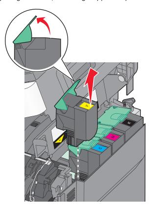
**5** Align the new toner cartridge, and then press down until it is all the way into the slot.
