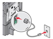
**3** Remove the plug from the printer EXT port  $\widehat{\mathbf{m}}$ .
