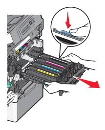
**8** Remove the used developer unit.
