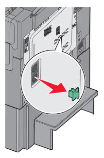
**4** Connect your telecommunications equipment directly to the printer EXT port : Use one of the following methods:
