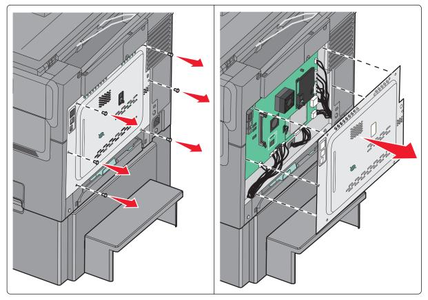
**Warning—Potential Damage:** System board electronic components are easily damaged by static electricity. Touch something metal on the printer before touching any system board electronic components or connectors.
