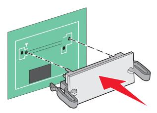
**Note:** The entire length of the connector on the card must touch and be flush against the system board.
