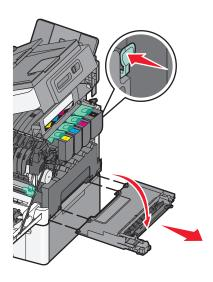
**5** Press the green levers on each side of the waste toner bottle, and remove it.
