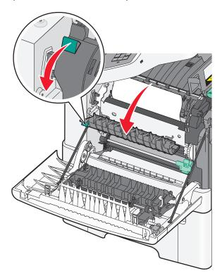
**3** Hold the fuser cover down, and then remove the jammed paper.
