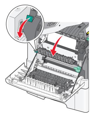
**3** Hold the fuser cover down, and then remove the jammed paper.
