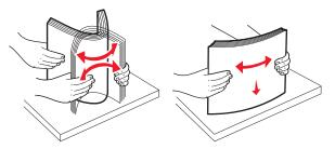
• Hold transparencies by the edges. Straighten the edges on a level surface.
