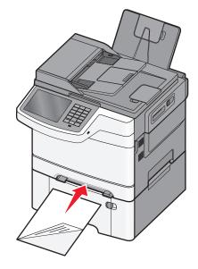
Note: Align the long edge of the sheet so that it is flush with the right side of the manual feeder.
