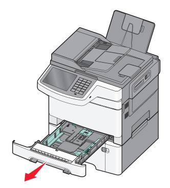
**2** Squeeze the length guide tab, and then slide the guide to the correct position for the paper size being loaded.
