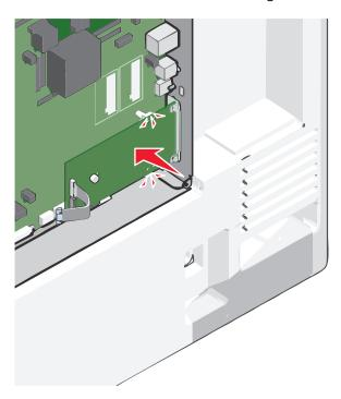
**9** Insert the long thumbscrew and turn it clockwise, enough to hold the ISP in place, but do not yet tighten the thumbscrew.
