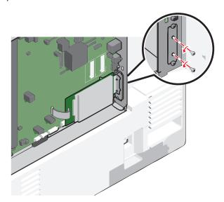
**b** Remove the screws attached to the printer hard disk mounting bracket, and then remove the bracket.
