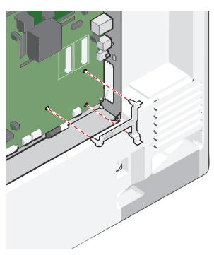
7 Install the ISP on the plastic tee. Angle the ISP over the plastic tee, and then slant it toward the plastic tee so that any overhanging connectors will pass through the ISP opening in the system board cage.
