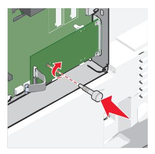
**10** Attach the two provided screws to secure the ISP mounting bracket to the system board cage.
