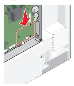
4 Remove the printer hard disk.
