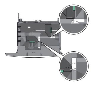
2 Squeeze and then slide the width guide to the correct position for the paper size you are loading.
