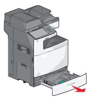
Notice the size indicators on the bottom of the tray. Use these indicators to help position the length and width guides.
