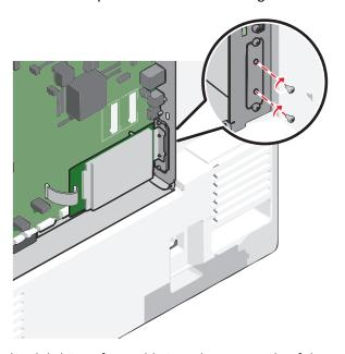
**c** Insert the plug of the printer hard disk interface cable into the receptacle of the system board.
