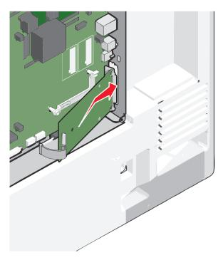
**8** Lower the ISP toward the plastic tee until the ISP is seated between the guides of the plastic tee.
