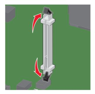
**4** Align the notches on the memory card to the ridges on the connector.
