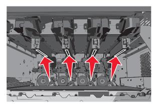
4 Clean the lenses using compressed air.
