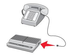
**5** Connect a third telephone cord from the answering machine to the EXT port  $\widehat{\ }$  of the printer.
