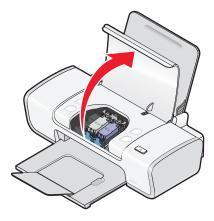
**3** Press down on the cartridge carrier lever to raise the cartridge carrier lid.
