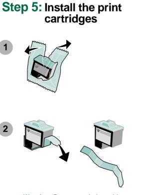
**Warning:** Do **not** touch the gold contact areas on the back and bottom of the cartridges.
