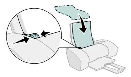
**Note:** A4 size paper should extend beyond the top of the paper support. Letter size paper should align with the top of the paper support.
