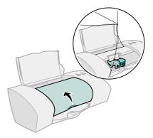
**Note:** The cartridge carrier moves to the loading position when you open the front cover.
