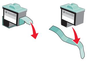
**Warning:** Do *not* touch or remove the gold contact areas on the backs and bottoms of the cartridges.
