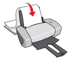
**Note:** Forcing the paper too far into the printer may cause a paper jam. For help, see "Printer has a paper jam" on page 61.
