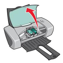
The cartridge carrier moves to the loading position, unless the printer is busy.
