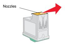
**d** Using another clean section of the cloth, gently hold the cloth against the contacts for about three seconds, and then wipe in the direction shown.
