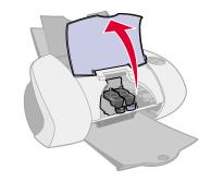
**b** Remove the cartridges.
