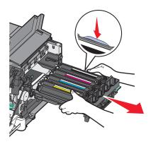
**8** Remove the used developer unit.
