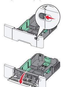
**2** Grasp the extension, and pull it straight out until it is fully extended.
