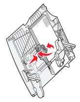
7 If you are loading a different type of media than was previously loaded in the tray, change the Paper Type setting for that tray on the operator panel.
