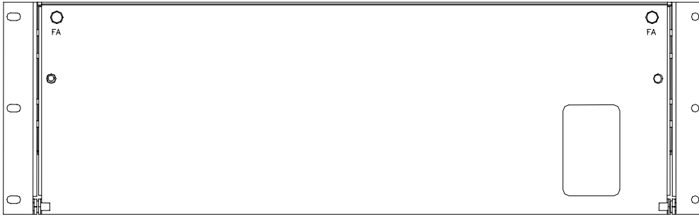
Figure 13 Front view of the (24) Plug-In 1-100 A circuit breaker panel
