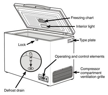
Before starting up the appliance, plug the defrost drain opening in the floor of the appliance with the plug provided. This is important to ensure that the appliance works properly.
