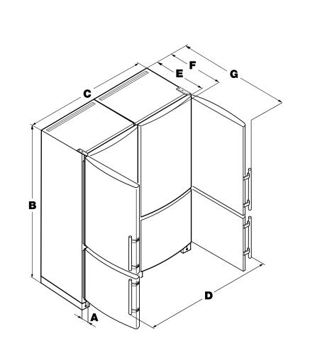
Overall height can be increased on SBS 32 units by 5/8" (16 mm) by adjusting the roller base.
