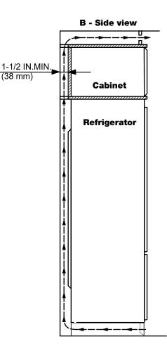
The refrigerator is designed to allow proper air flow when the appliance is installed up against the wall.
