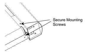
**6.** Repeat steps for opposite side. After completion run treadmill and check for interference or binding. If needed loosen Mounting Screws, re-align Guard, and refasten securely.
