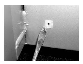
NOTE: Do not replace washer. Having a washer and the grommet will raise the guard too high and cause rubbing against the belt resulting in premature wear and reducing belt life.
