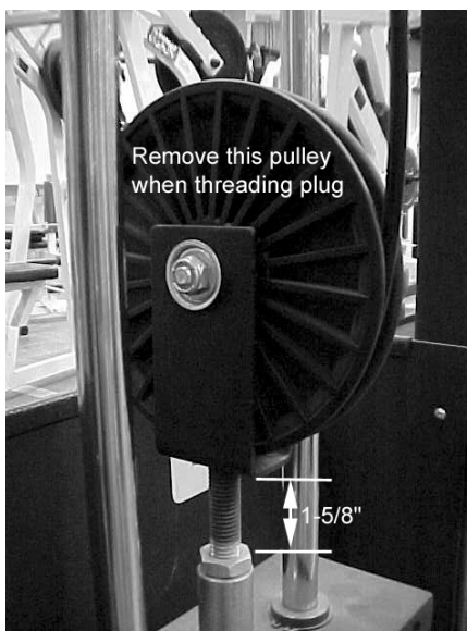
Figure 9. Bolt the floating pulleys into the 190 lb weight stacks.
