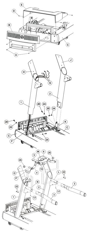
**9.** Position the right end of the ERGO FRONT CROSSBAR (#4) near the large access hole on the inside of the RIGHT UPRIGHT HANDLEBAR BRACKET (L).
