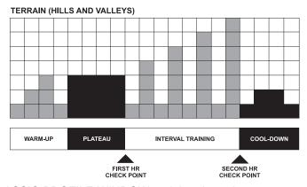
Each column, as seen in the CLASSIC PROFILE WINDOW and the chart above, represents one interval. The overall duration of the workout determines the length of each interval. Each workout is made up of 20 intervals, so the duration of each interval is equal to the duration of the entire workout divided by 20.
