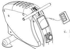
c. Push the display console into the hole in the in the main frame until secure.
