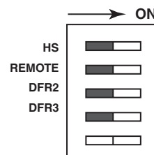
Figure 2 - Contractor adjusted setting for STANDBY
