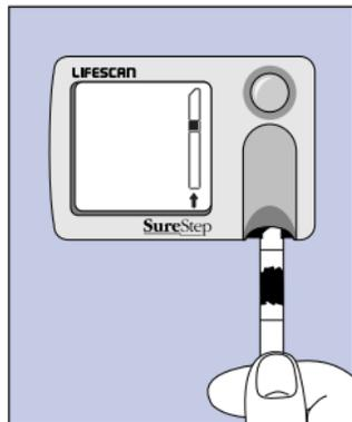
**CAUTION:** *If you do not firmly insert the test strip into the meter until it stops, the test may start but you may get an inaccurately low result. Do not remove test strip until countdown is complete.*
