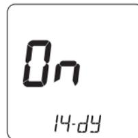
For accurate 14-day and 30-day blood glucose averages, you must mark control solution test results by pressing the green **C** button again while the glucose level is displayed. This will keep them from being included in your blood glucose test averages. If you wish to turn the averages off, press the green button. The following display will appear:
