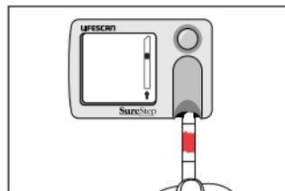
**4** Firmly push the test strip into the test strip holder, with the tapered-end first and the confirmation dot facing down, until it stops. Read result. Do not remove strip until countdown is complete.
