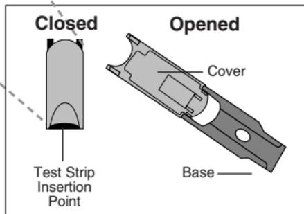
The cover protects the lens area and the base holds the OneTouch® SureStep® Test Strip.
