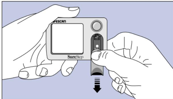
2. Wipe the test strip holder gently with a cotton swab or soft cloth dampened with water. Thoroughly wipe the grey area on the inside cover. Clean both sides of the test strip holder base, especially around the hole. **Dry the test strip holder completely with a soft cloth or lint-free tissue.**
