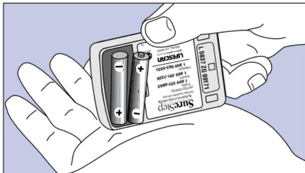
4. Insert two new AAA alkaline batteries, matching the + end of each battery with the + sign in the battery compartment.
