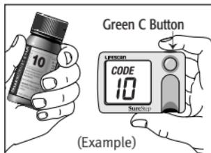
**4** Compare the code number on the meter to the code number on the test strip vial. If the code numbers do not match, press the green **C** button until the code number on the meter matches the code number on the test strip vial.
