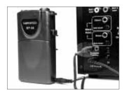
3 The battery charging indicator LED (labeled CHARGING) lights green when the Transmitter is connected with a charging cable to the TRANSMITTER CHARGING jack on the back panel of the Receiver/Amplifier. When charging is complete (8-12 hours), the CHARGING indicator light will turn off.
