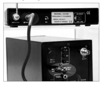
A 1/4" phone-to-RCA cable is used. The 1/4" phone plug goes into the AF OUT jack on the back of the CX-50. The RCA plug is inserted into AUXILIARY INPUT jack on the Receiver/ Amplifier. For the best sound quality, the volume adjustment on the front of the CX-50 should be turned clockwise as far as it will go. Depending on which AUX INPUT jack is selected, the audio output is adjusted using AUX1 or AUX2 VOLUME controls on the front of the Receiver/Amplifier.
