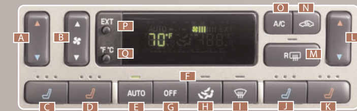
DUAL AUTOMATIC TEMPERATURE CONTROL (If Equipped)
