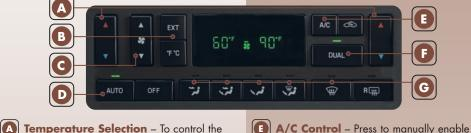
temperature for the driver and for the passenger, select the desired temperature by pressing the driver's or passenger's temperature control.
