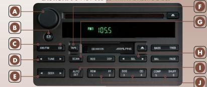
**Nolume/Power Control** – Press the control to turn the audio system on or off. Turn the control to raise or lower volume. To engage speed sensitive volume feature (if equipped), press and hold the volume control for five seconds (with the radio on), then press SEL to choose the compensation level.
