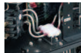
Electrical Connections coated with protective compound for long-term reliability in harsh environments.
