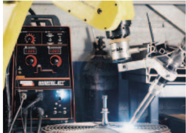
The STT Waveform controls heat input and reduces spatter and fume
