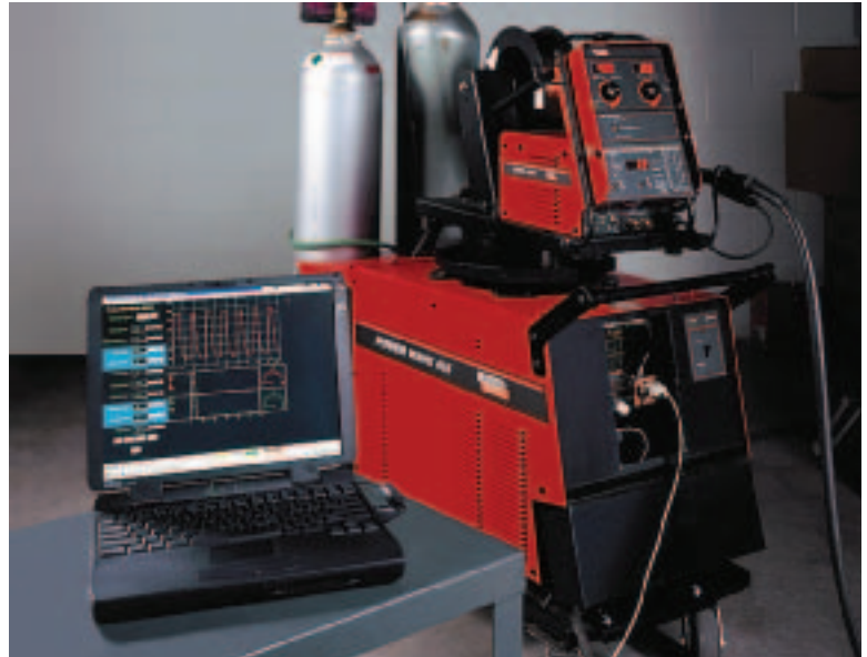
Alterations to the waveform can be made during the weld, using software created by Lincoln Electric.
