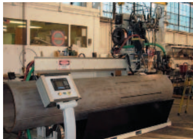
AC/DC Submerged Arc uses Waveform control for infinite phase-shifting to accommodate up to 5 arcs without arc blow
