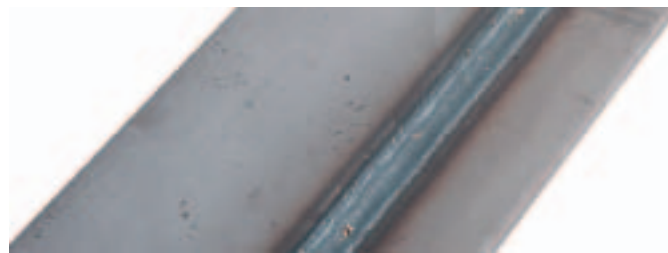
3/16" (4.8 mm) Horizontal Lap Weld
