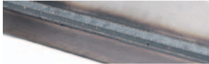
This thin gauge lap weld was made at a travel speed of 100 ipm
