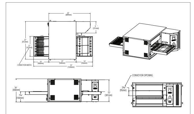
**ELECTRICAL SERVICE:** Heat is supplied by six (6) infrared elements at 1200W each, (user may select any three (3) elements to be activated at one time,) one (1) main fan element at 8000W. Each finisher is rated at 12 kW. The DTF-16 is available in 208V or 240V, 3-phase power. A separate circuit breaker is required for each finisher with the proper voltage, amperage, phase and hertz as indicated by model number. UNIT REQUIRES 50 AMP SERVICE. Plug type NEMA-15-50P.
