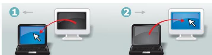
B. The Picture in Picture (PIP) mode is the value added to this device and is suitable for a single display monitor.
