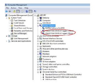
You can also check the installation under **Universal Serial Bus controllers**, this should show one new device.
