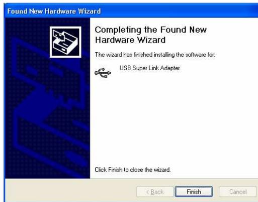
5.7.10 Plug the USB 2.0 Link cable into a USB Port, , the pc will detect and install a new item “**USB SuperLink Adapter**” at “**Universal Serial Bus controllers**” of “**Device Manager**”.
