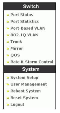
The function menus contain two parts: **Switch** for setting up the switch functions and **System** for maintaining the system parameters.
