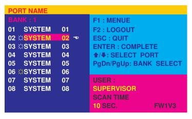
Use the cursor keys to select the computers connected on bank 1. Select the computer by pressing the ENTER key. This symbol indicates all active computers connected. Computers connected not showing this symbol may be either be switched off or in a standby mode. To access ports between 9...16 simply scroll down below port 8
