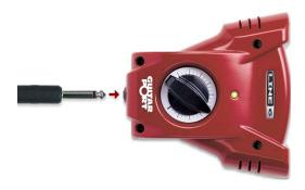
**Instrument input** - your electric guitar or bass, plug it into one of these inputs using a standard 1/4-inch TS instrument cable. This inputs the signal into GearBox where you can choose your Tone and route the processed signal both to your audio software and out the GuitarPort outputs.
