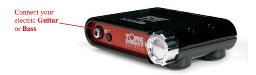
**Guitar/Bass** - To input your electric guitar or bass, plug it in here using a standard 1/4-inch TS instrument cable. This input also features a **Pad switch**; engage this switch when using a guitar/bass with high-output or active pickups, to avoid overdriving the input.
