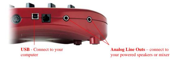
**Analog Line Outs** - These Left and Right <sup>1</sup>/<sub>4</sub>-inch jacks output all audio signals; the audio from your audio software on the computer, and anything plugged into any the Instrument input. So,
