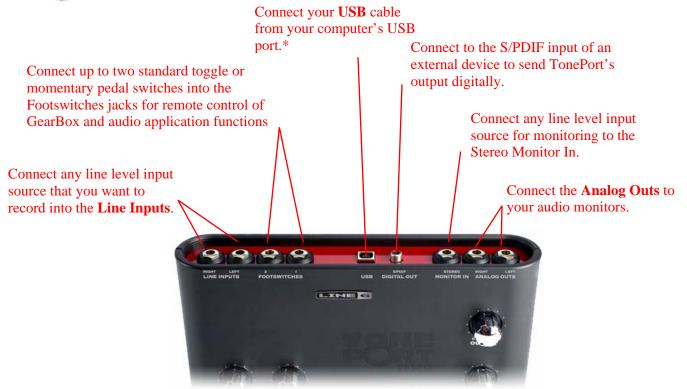
\*Note – be sure to always **power off** or **mute** your speakers or monitoring setup *before* connecting and disconnecting the USB cable between TonePort and your computer, as well as before booting up or shutting down your computer if TonePort is already connected. The best practice is to always power on your speakers last, and power them off first when connected to other audio gear to avoid a "pop".
