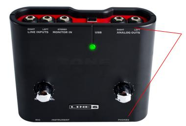
Connect the mono 1/4-inch Analog Line Outputs . Or, connect a 1/4-inch stereo cord to the **Headphone Out**
