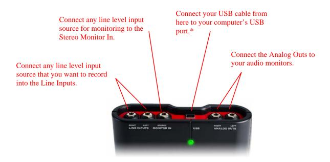
\*Note – be sure to always power off or mute your speakers or monitoring setup before connecting and disconnecting the USB cable between TonePort and your computer, as well as before booting up or shutting down your computer if TonePort is already connected. The best practice is to always power on your speakers last, and power them off first when connected to other audio gear to avoid a "pop".
