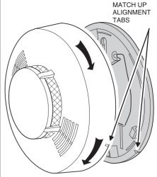
TWIST SMOKE ALARM CLOCKWISE TO LOCK TO MOUNTING PLATE
