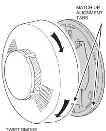
ALARM CLOCKWISE TO LOCK TO MOUNTING PLATE
