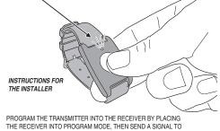
PROGRAM THE TRANSMITTER INTO THE RECEIVER BY PLACING THE RECEIVER INTO PROGRAM MODE, THEN SEND A SIGNAL TO THE RECEIVER FROM THE TRANSMITTER. REFER TO THE ULLISTED PERS-2400B OR PERS-3600B RECEIVER'S PROGRAMMING INSTRUCTIONS FOR DETAILS.
