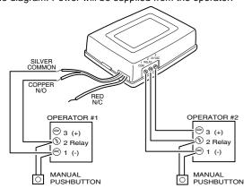
**DESCRIPTION:** The Delta-3 DR-2 digital receiver is a two-channel wireless radio control designed for use with automatic garage/gate operators and access control systems. The receiver can be activated by any of the Delta-3 format transmitters. **Receivers must be mounted at least 8 feet apart.**
