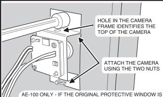
DAMAGED, IT MAY BE REPLACED BY PRESSING IT OUT FROM THE OUTSIDE IN. REMOVE THE ADHESIVE BACKING FROM THE NEW WINDOW (INCLUDED) AND PRESS IT INTO PLACE. ADHESIVE TOWARDS THE FRONT.
