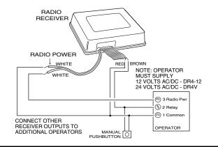
**DESCRIPTION** The Delta-3 DR4V & DR4-12 digital receivers are four-channel wireless radio controls designed for use with automatic garage/gate operators and access control systems. The receivers can be activated by any of the Delta-3 format transmitters. **Receivers must be mounted at least 8 feet apart.** The Delta-3 radio format provides 256 different digital codes. The
