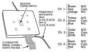
**STEP 4A** Connecting receiver (using transformer power). A Model T12A (used with DR4-12) or 524 (used with DR4-V) transformer can be used to power the receiver when connecting receiver to any operator. Connect as shown, then plug the transformer into a convenient (unswitched) 120 VAC outlet.
