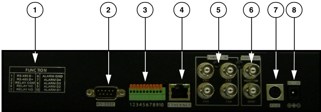
1. **ALARM BLOCK CHART** - Outlines the Alarm Block connections
