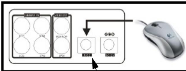
**USB Connection** - A mouse can be connected to the PS/2 Port on the back of the unit.
