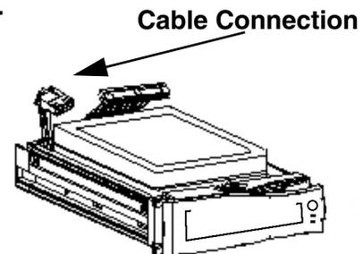
**STEP 4: Secure the Hard Drive in the Casing**
