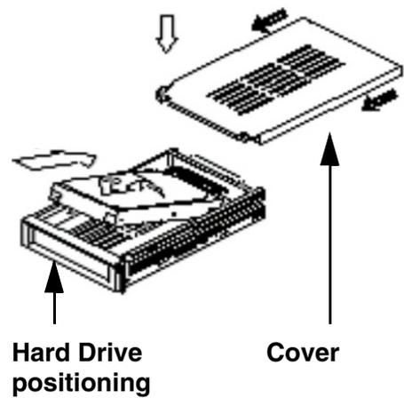
**STEP 6: Reinsert the Cartridge Casing into the DVR**
