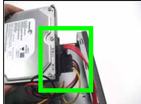
Figure 27.4 Connect the power and data cables.
