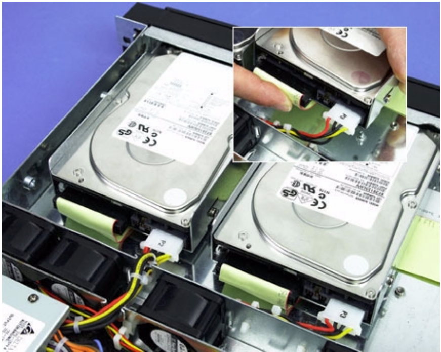
Figure 14 Drive Bay Installation
