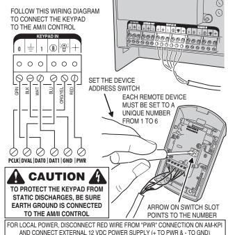
7. CONNECT THE CABLE & SET THE DEVICE ADDRESS
