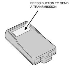
PRESS BUTTON FOR A MINIMUM OF 2 SECONDS
