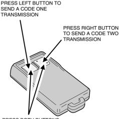
PRESS BOTH BUTTONS TO SEND A CODE THREE TRANSMISSION
